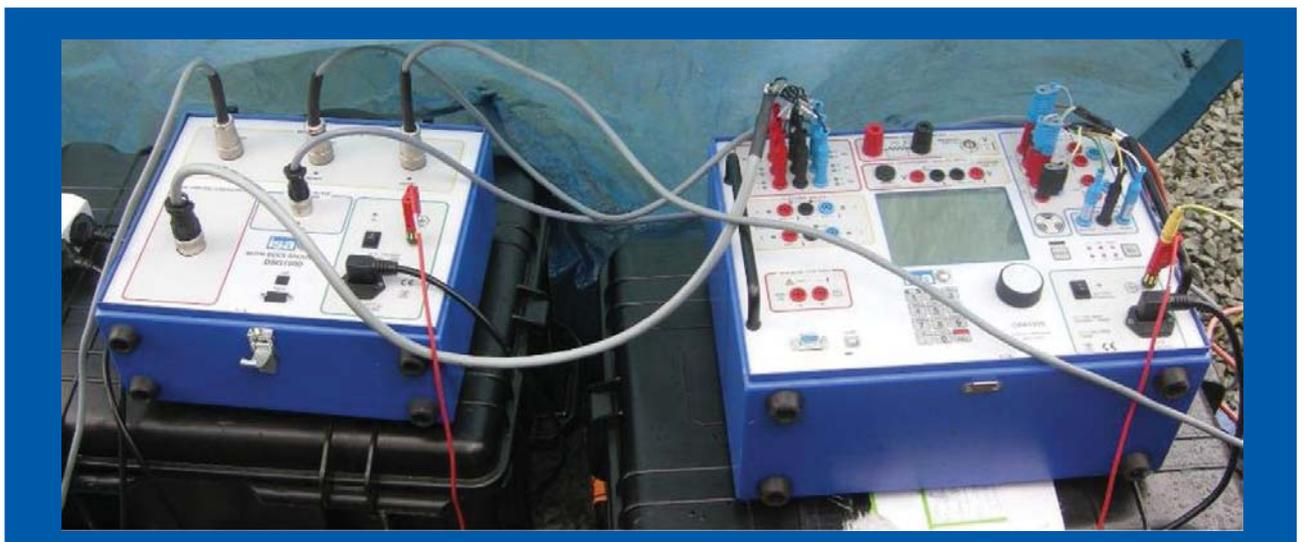
6. BSG 1000 connected to CBA 1000 during a test in a substation
