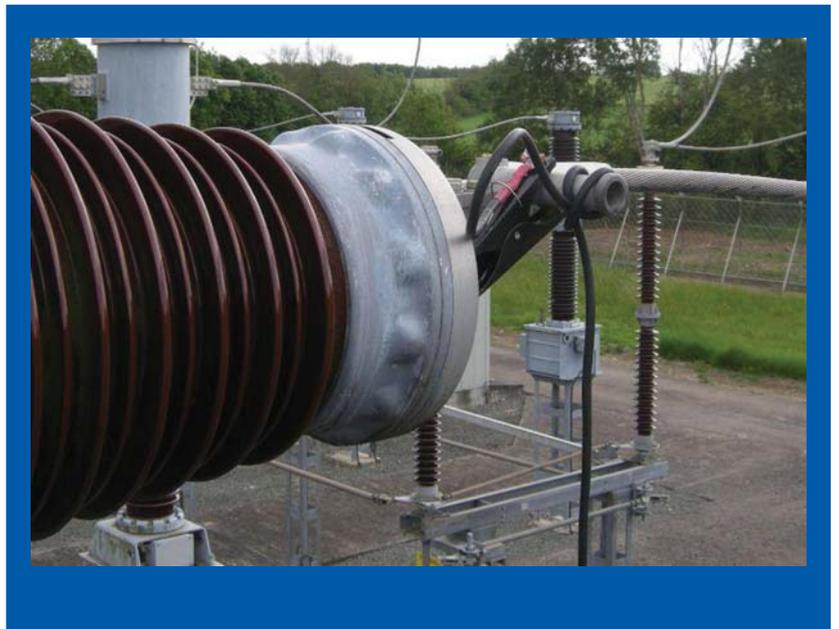
9. Clamps terminated by crocodiles supplied with BSG 1000, in action during a real test
