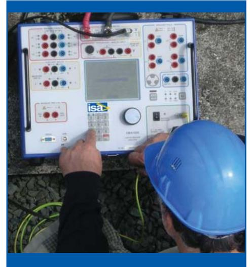
7. Operator using CBA 1000 in a substation test
