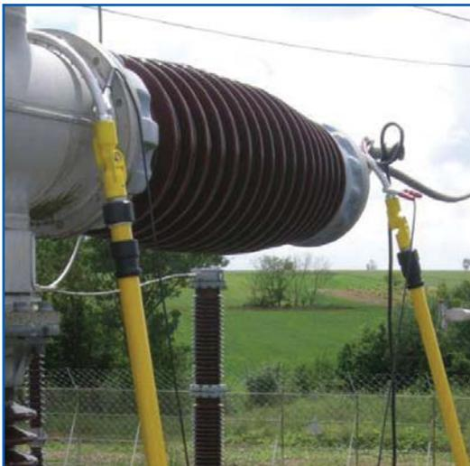
12. Arc clamp mounted on a real circuit breaker (with telescopic cranks)
