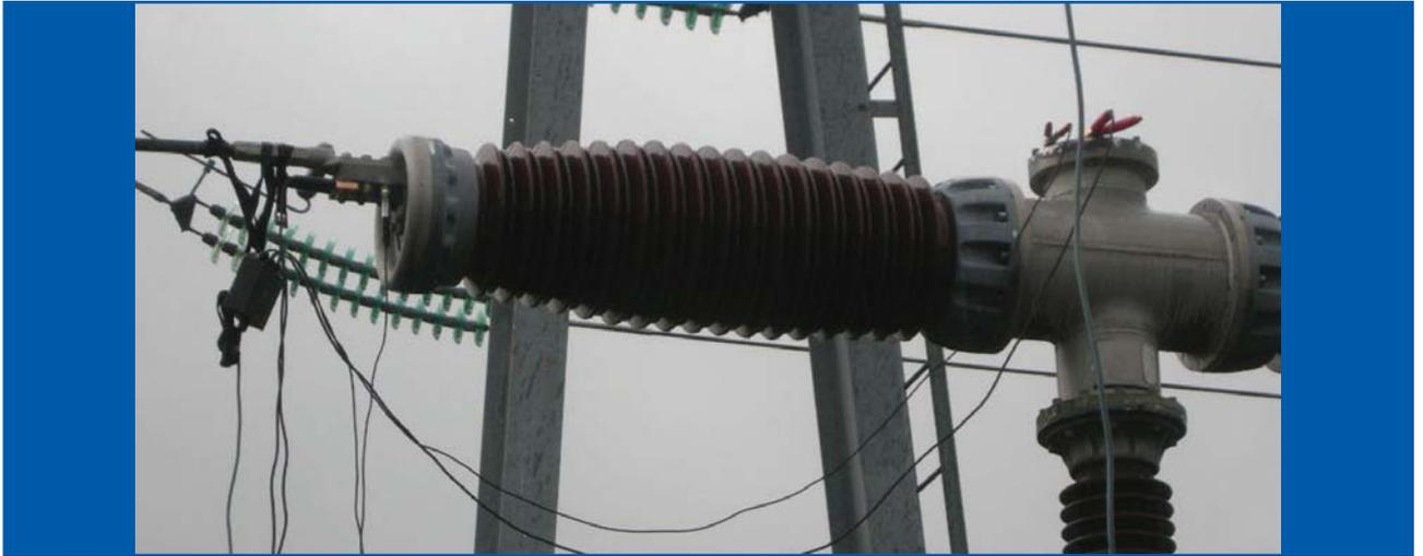
8. BSG remote head connection to a circuit breaker by crocodile clamps
