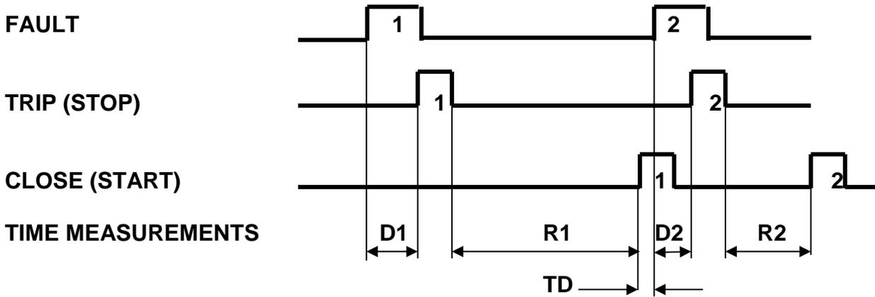
**Figure 4: Measure of Delay and Close times**
