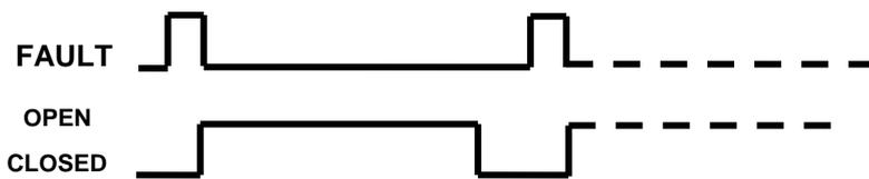
In this test mode the test set is edge triggered; the CB position is connected to the STOP input, and, from the Closed – Open position, the test set derives the fault generation commands, to perform the test as above.
